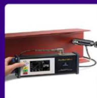
Dolly Pull Off Test - Hardness Test - ASTM D4541
