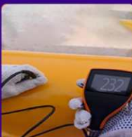
Dry Film Thickness - ASTM D7091 / ISO 19840
