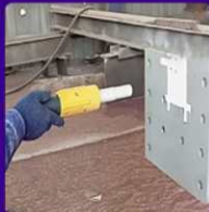
Blotter Test - ASTM D4285
