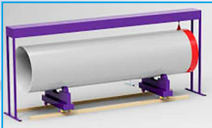
Reciprocator based External Rotating Pipe Coating
