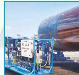
External Automatic Pipe Coating
