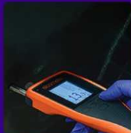
Air & Dew Point Temperature Meter: Relative Humidity Meter - ASTM E 337
